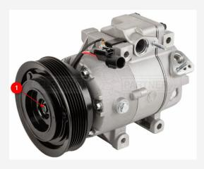
You have to note that the voltage drop does not exceed 0.5V in the wires to the compressor. Measure this while the compressor is activated.
