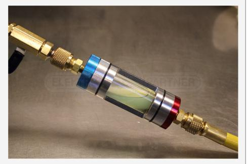
Gel-like, crystallised texture: Leak stop agent of poor quality, which reacts with refrigerant oil or leak detection agent. They forgot to create a vacuum before using leak stop agent.
