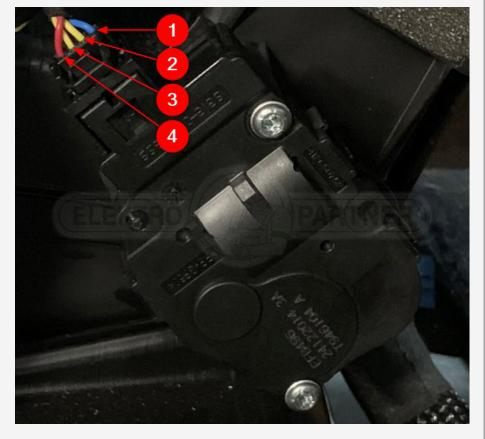
The resistance between pin 2 and 3 must be higher than 20 Kohm.
