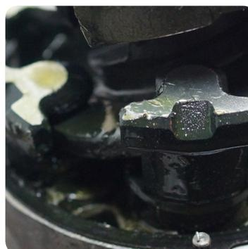
Crystallized leak-stop agent thickened the oil, creating visible snots on wobble plate and pistons
