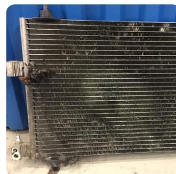
Seems tight, however, a condenser in such a condition cannot perform well and must definitely be replaced
