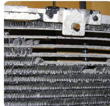
Several rows of missing fins caused by condenser corrosion
