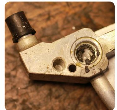
*Visible soiling at the condenser inlet.*
