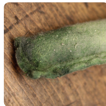
Worn out insert bag dryer - desiccant soaking by too much UV agent added to the system
