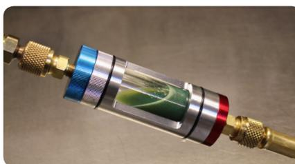
**TIP:** Use a supplementary glass inspection tool to spot possible contaminants circulating in the loop. This low-cost and useful tool is highly recommended for an effective system contamination diagnostic, performed in various situations: before, during and after flushing.
