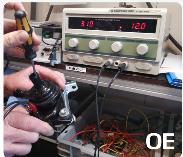
OE WATER PUMP The OE water pump is not equipped with a failsafe mode. This means that it will the amps will remain high and the temperature of the water pump will increase and in worst case overheat.
