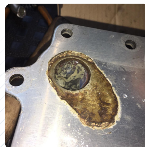
Lubricant mixed with coolant, seen on the oil cooler outlets. One of the most common outcomes of lubricant overpressure and internal bursting of the oil cooler.
