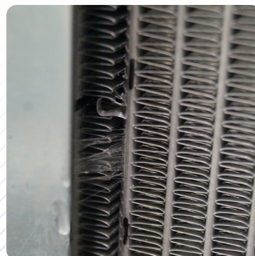
The outermost radiator tubes are often the first elements that burst due to excessive vibrations caused by missing or broken fitting bushings.
