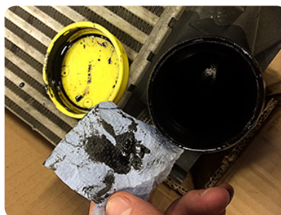
Oil residues clogging the intercooler, resulting in a dysfunctional intercooler.
