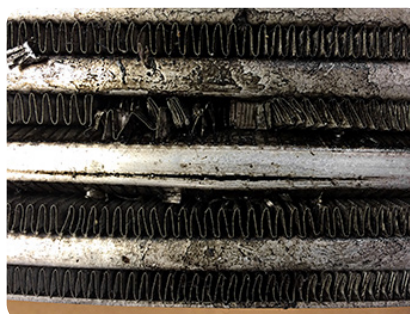
Fins are destroyed due to pressure failure. This error is often ascribed to an error in the tubes. However, the excessive amount of oil on the intercooler indicates a system pressure failure.
