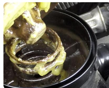
Impaired oil separator of the crankcase ventilation system.
