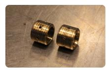
**Oil contamination:** The clearly visible grooves on the journal bearing surface arise from frictions and excessive material abrasion provoked by impurities in the oil. Despite the presence of oil, shaft of this turbo get seized.
