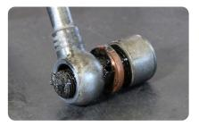
**Oil supply disturbance:** Severe oil contamination (sludge/carbonizing) caused oil feed line restrictions visible on banjo fitting.
