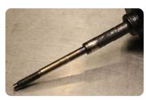
**Insufficient Lubrication:** The surface of the turbo shaft is black and carbonized. Insufficient oil supply have caused overheating at first, thus making the steel color change. The blueish-to-yellowish color temperature is a heat tint caused by overheating of the shaft steel. Next, the remaining oil will start coking on the surface, making the black sinters.
