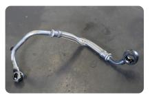
Oil supply disturbance: Oil feedline deformation caused by careless installation. The line is tight but the deformation caused oil thus shortages in lubricant supply to the turbo.
