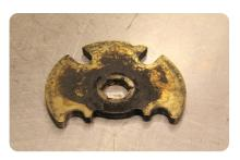
**Insufficient lubrication:** Oil coking on the thrust bearing – failure provoked by insufficient lubrication that caused overheating.
