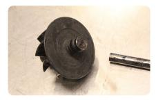
**Insufficient Lubrication:** Broken shaft caused by lack of Lubrication. The high rotation speed and frictions within the moving parts have caused the temperature to increase extremely, the shaft to warm up, and ultimately break by seizing.
