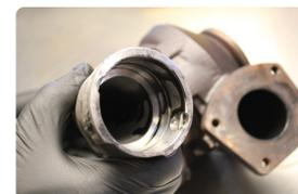
Oil contamination inside is a sign of leaking oil seals. They occur as the shaft moves back and forth. In the end, the shaft may break totally too.
