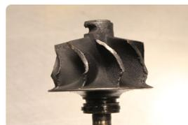
Torn out compressor/turbine wheel blades – outcome of and excessive shaft play / broken thrust bearing.
