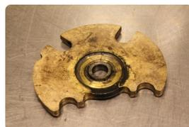
Visible grooving on the thrust bearing - outcome of an excessive thrust pressure affecting the turbo.
