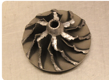
Compressor wheel damage caused by foreign objects. The blades have been hit repeatedly, and the compressor housing inducer will also bear signs of hits by the foreign objects.
